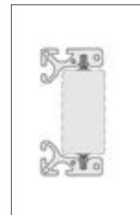
To construct a linear guide, two centric (fixed) and two eccentric (adjustable) bearing units are normally required. Each pair of single bearing units can be replaced by one double bearing unit.
