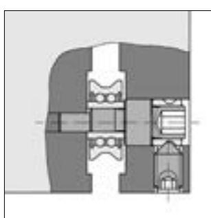
The eccentric bearing units must be set prior to the guide carriage being used:
