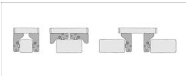
The roller profiles provide a variety of fastening options using the grooves of Line 8 Profiles, this greatly simplifying installation and alignment on profiles or carriage plates.
